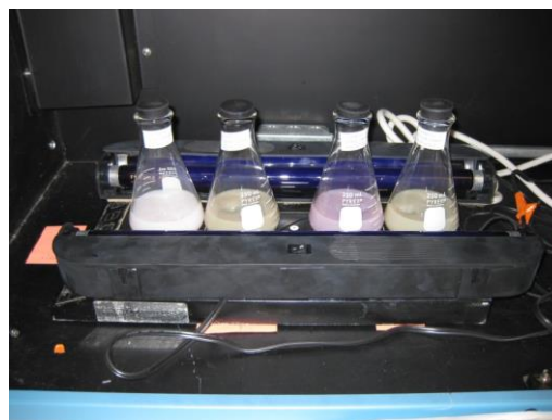
Figure 2: Photodeposition preparation method for quantum dot formation on TiO 2 .
